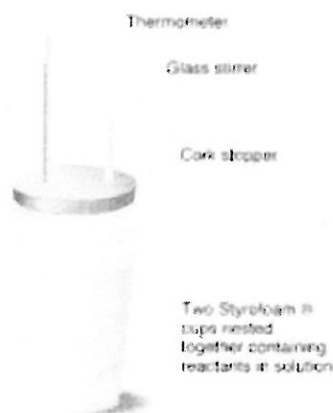
Figure 1: Diagram of a Simple Calorimeter
