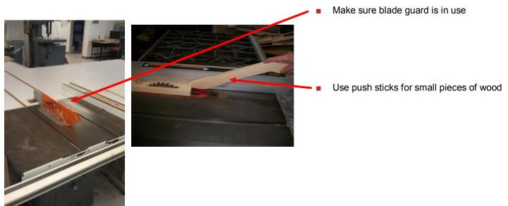
Severe cuts and amputations to the fingers or hands can occur if the operator contacts the saw blade.
