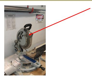
Make sure self-adjusting blade guard is in use
