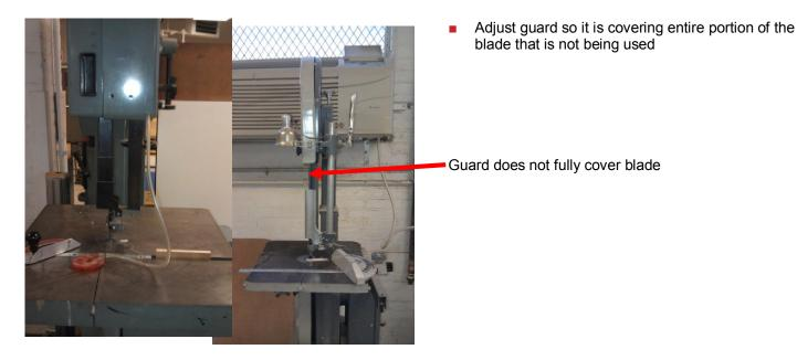
Serious cuts or amputations can occur if the operator contacts the blade. Extreme caution is necessary because the operator's hands may come close to the saw blade — and a band saw cannot be fully guarded.
